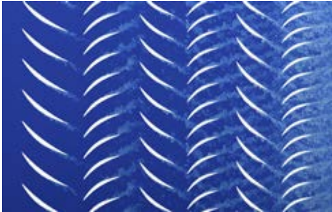
FIGURE 17 : ENTROPY CONTOURS PROGRESSING THROUGH THE 3-STAGE COMPRESSOR CREATE2BIS
