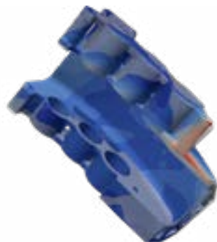
FIGURE 9 : POST BUILD DISTORTIONS OF A 3D PRINTED BRAKE CALIPER - COURTESY OF ANY-SHAPE
